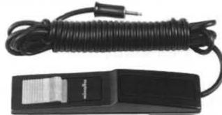
This 3m (10 ft.) cord serves with the electromagnetic shutter release system in place of a cable release as well as for positive unfailing remote control. It plugs into the remote-control jack provided on the camera and is used to avoid camera movement in single-frame and tripod filming. A built-in lock device enables continuous-run filming.
