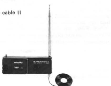
This small unit has a tuning dial and antennas and is directly connected to the sound system when conveniently attached on the side of the camera. The U.S. model can be used to record music or speech from FM broadcasts or mix them with input from the microphone jack for the soundtrack. It is also used to pick up sound for recording from the U.S. model wireless FM microphone. The European model is for use with the special frequency European microphone.
