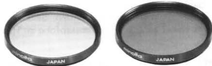
These have 46, 49 and 62mm — diameter threads to fit the screw mounts of the XL 42, 64, and 84 lenses, respectively. The UV filter cuts ultraviolet light and can be used to protect the lens; the 4X ND (neutral-density) reduces scene light passing through the lens by two stops to 1/4; the 1B is used for improving bluish rendition of subjects in shade illuminated by blue sky, on overcast or rainy days, or obscured by atmospheric haze.
